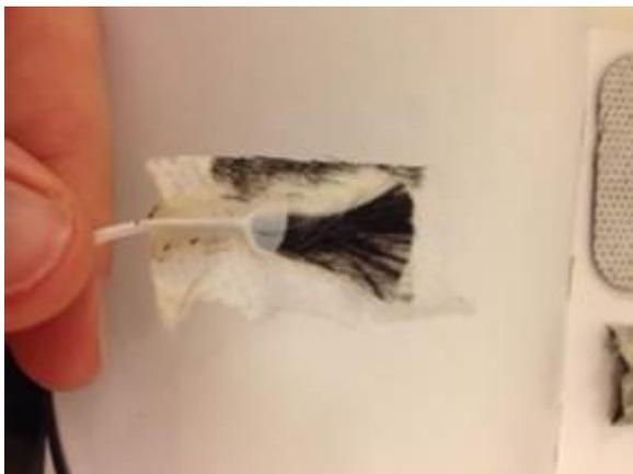
3. Carefully peel away the carbon fibres and the lead attached to them from the rest of the electrode so you're left with something like this.
