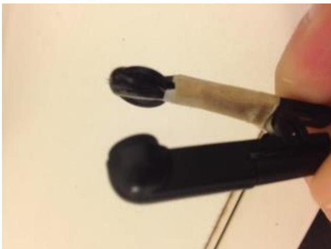
6. The carbon fibres will stick out a bit beyond the auricular clip: take a small strip of masking tape and carefully tape the fibres to the back of the auricular clip.
