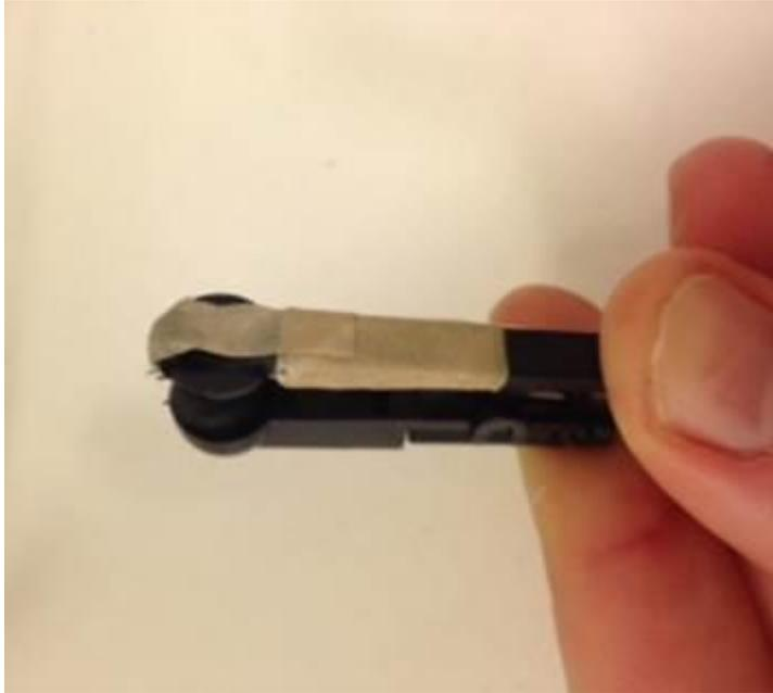
7. Attach the leads of the auricular clip to the V-TENS machine. The V-TENS should have two separate black leads that plug into the two output channels on the device (as shown). Each of these leads has a black and a red end which you use to attach to one auricular clip.
